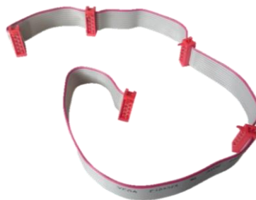
Figure 10: PoExtension2 cable for connecting PoStep drivers with PoKeys57CNC device
